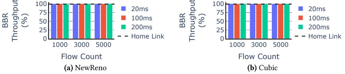
Figure 3.8: BBR takes 99.9% of total throughput when competing with an equal number of NewReno or Cubic flows.
