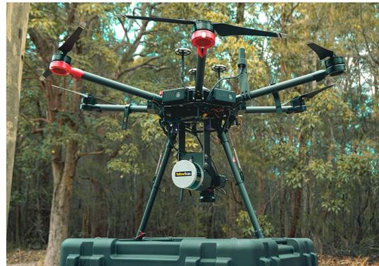
(d) The DJI Matrice 600, released in 2016, is a fully-programmable autonomous drone with support for native onboard GPUs. Its huge size limits practical deployment [36].
