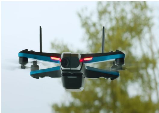
(c) The Skydio 2 platform, released in 2019, provides a small set of semi- and fully-autonomous capabilities like person tracking and obstacle avoidance [110, 111].
