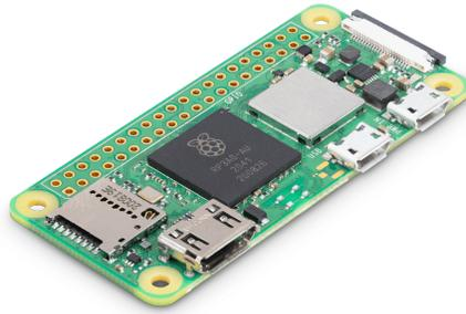
The Pi Zero 2 W is 16 g but lacks cellular connectivity and requires an external power source.
