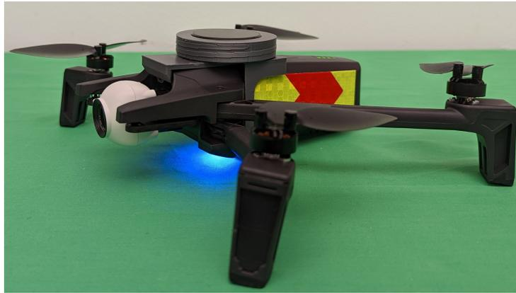
Figure 3.6: Drone with Watch-Harness Payload
