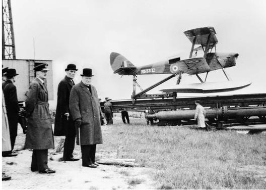
(a) The British-made "Queen Bee", introduced in 1935, was one of the first radio operated aircraft and served as an anti-aircraft practice target [70].
