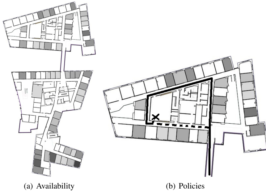
Figure 3.3: (a) We measured the availability of occupants in each of 78 offices in our building - darker gray represents higher availability. (b) The OPOMDP policy takes the shortest path to the lab (dashed line) while the optimal HOP-POMDP policy takes a longer route with more available people (solid).
