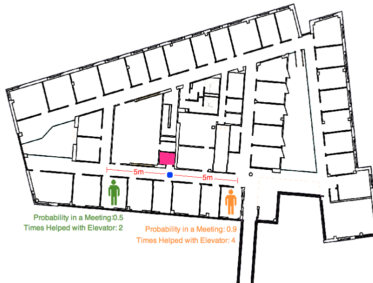
Figure 5.2: Participants were shown an image with two humans (orange and green) in different offices or locations and different state attributes and asked which they thought the robot (blue dot) should navigate to to ask for help using the elevator (pink square) or coffee maker.
