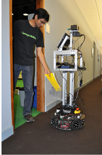
Figure 2.1: CoBot stops at a room to pick up a folder before navigating autonomously to drop it off (Biswas and Veloso (2010); Biswas, Coltin, and Veloso (2011)).
